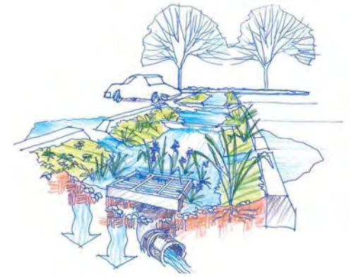
A bioswale is used to slow the speed of surface runoff to allow the stormwater to infiltrate back into the ground.
