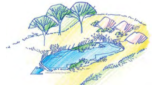
Naturalized detention is used to temporarily store storm stormwater on site and release it at a controlled rate.
