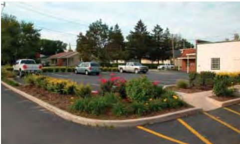
Parking lot landscape islands provide safe pedestrian access.
