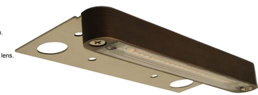
Crafted from cast brass, the Timberline hardscape light features a highly efficient embedded 4-watt, warm-white LED array (251 lumens). It can be mounted under a horizontal cap or flush to a vertical or horizontal surface. Clear and frosted high-impact lenses included. Five-foot factory-installed 18/2 wire lead.
