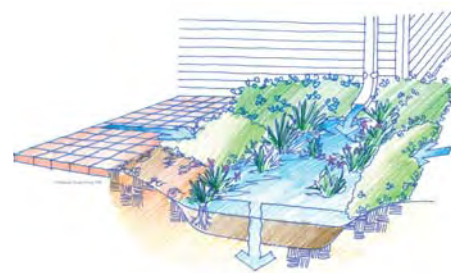
Rain gardens slow the stormwater runoff from impervious surfaces to allow infiltration back into the soil.
