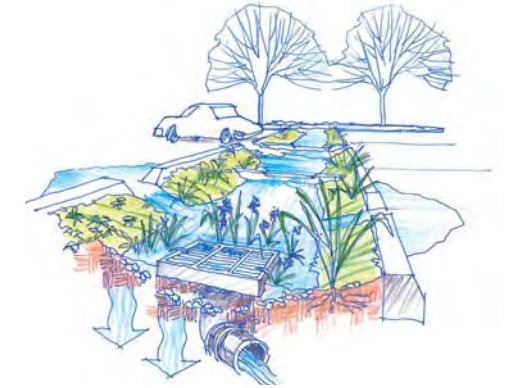
A bioswale is used to slow the speed of surface runoff to allow the stormwater to infiltrate back into the ground.
